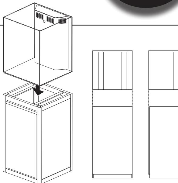
Place the aquarium (15) on the cabinet, make sure the tank is aligned with the cabinet.
