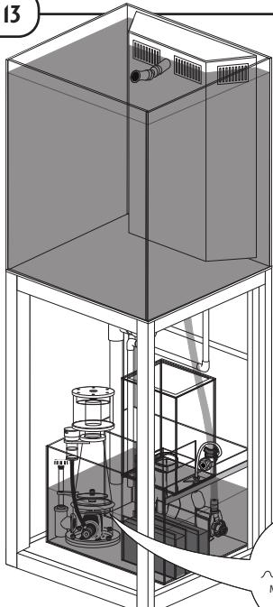
Open the tap of the transit pipe and fill the tank until the maximum water level has been reached in the sump.
