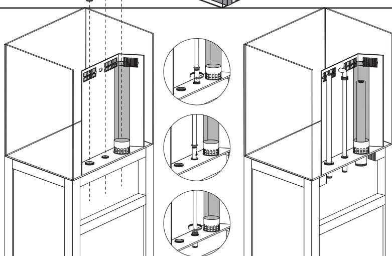
Place the transit pipe (1), the outflow pipe (4) and the overflow pipe (6) in the slots.
