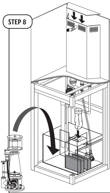
Place the filter-sock (18) and the skimmer (7) in the appropriate sections of the sump.
