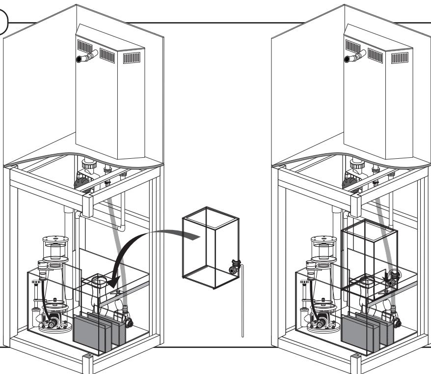
Place the water reservoir (17) on the sump. Connect the float hose (11) to the float.
