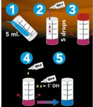
Professional drip test for precise determination of GH - total hardness in ponds.
