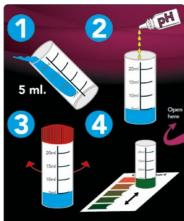
Professional drip test for precise determination of pH - acidity in ponds.
