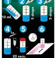
Professional drip test for precise determination of NO<sub>3</sub> - nitrate value in ponds.
