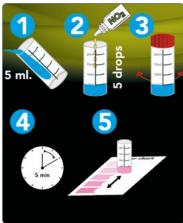
Professional drip test for precise determination of NO<sub>2</sub> - nitrite value
